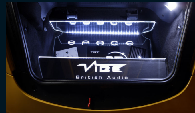
ONE SMALL BOOT FITS ALL Three amps, a multichannel audio processor and a line output converter
