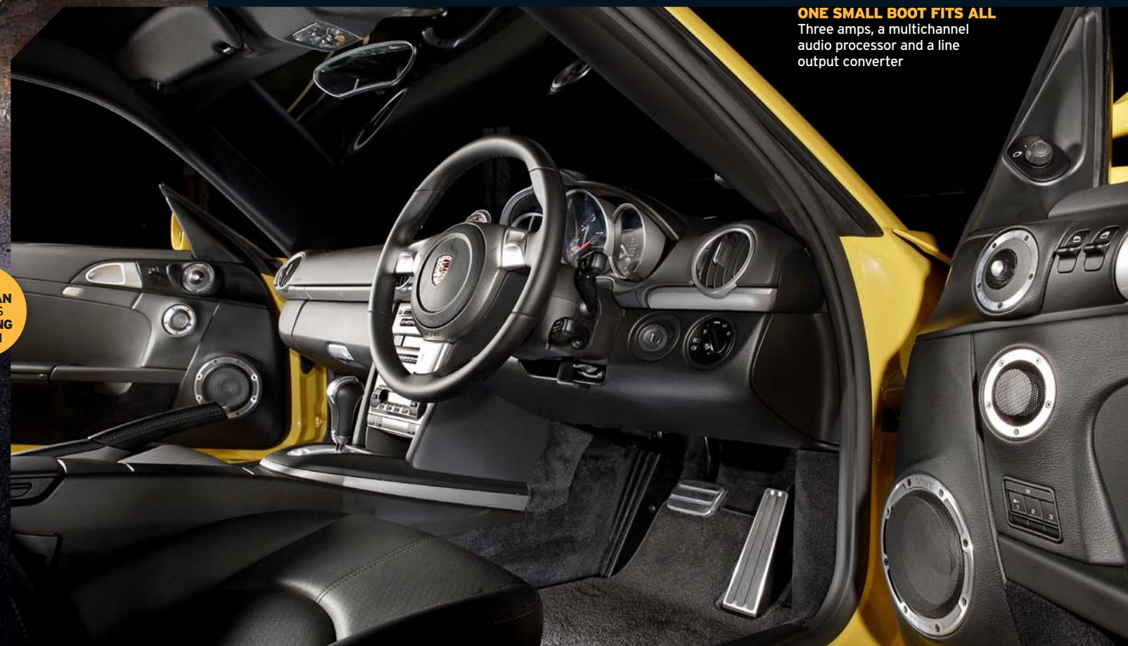
SOUND INSTALL. Tweeters, mid rangers and woofers are beautifully integrated into the door panels
